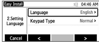
**3** After selecting the setup method, press the **[Next]** soft button. Depending on the selected setup method, the easy installation step is changed.
