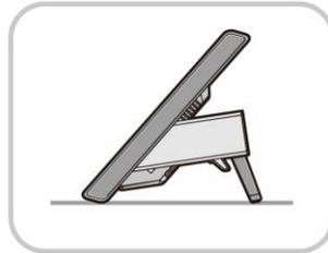
**1** Fix one latch of the cradle to the top or bottom groove of the phone.
