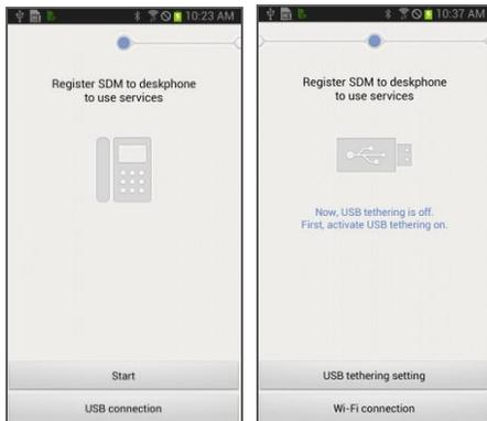
3 Turn on USB tethering by selecting USB tethering setting at the bottom and select the Back button.
